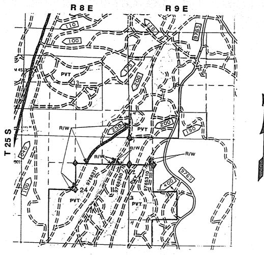
Road 9768250 - Begin ROW 640' (M), North from the South East Corner Sec. 13; End ROW 550' (SC), East from the CN 1/4 Corner Sec. 24. Also, Begin ROW 75' (M), North from the Center 1/4 Corner Sec. 24; End ROW 40' (M), West from the Center 1/4 Corner Sec. 24
